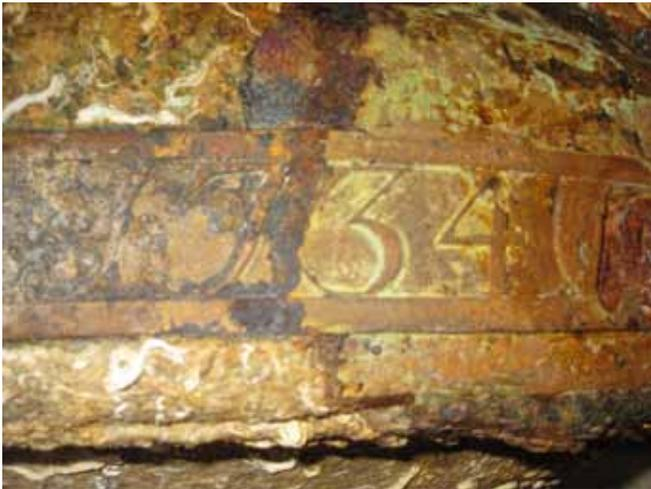
Fig. 7. The date of '1734' on the base ring of 12-pounder cannon C28.
